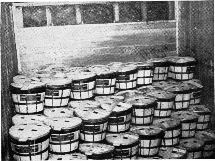
FIGURE 19.—Partial load of \frac{1}{2} -bushel baskets in a refrigerator car.
